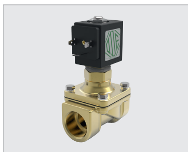
21HT5ZOY160-BDA230AC-305, 2-weg magneetventiel 3/4", NO, 230 V AC, 8 W, NBR
