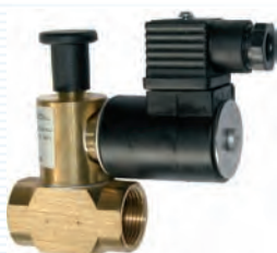
Electrovanne TV EVG 001 12 V DC, raccord 3/4", comportement NO, PN = 500 mbar
